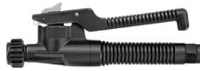
TriggerJet® Pressure: 150 psi (10 bar) Capacity: 2 gpm (7.6 l/min) 1/4" or 3/8" hose or 1/4" NPT or BSPT (F) inlet conn. 11/16"-16 UniJet THD outlet conn.
