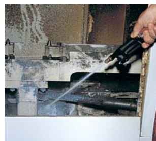
TriggerJet spray gun used to clean machining centers.
