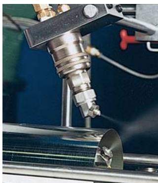
28JJAU automatic spray gun used in can coating application.
